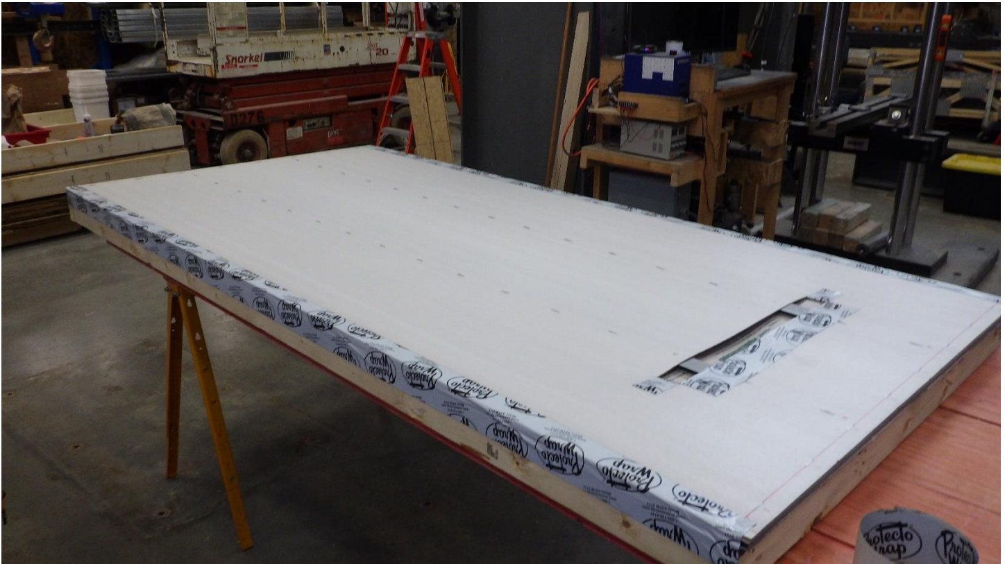
Figure 3: Test Specimen with Slot Fault
